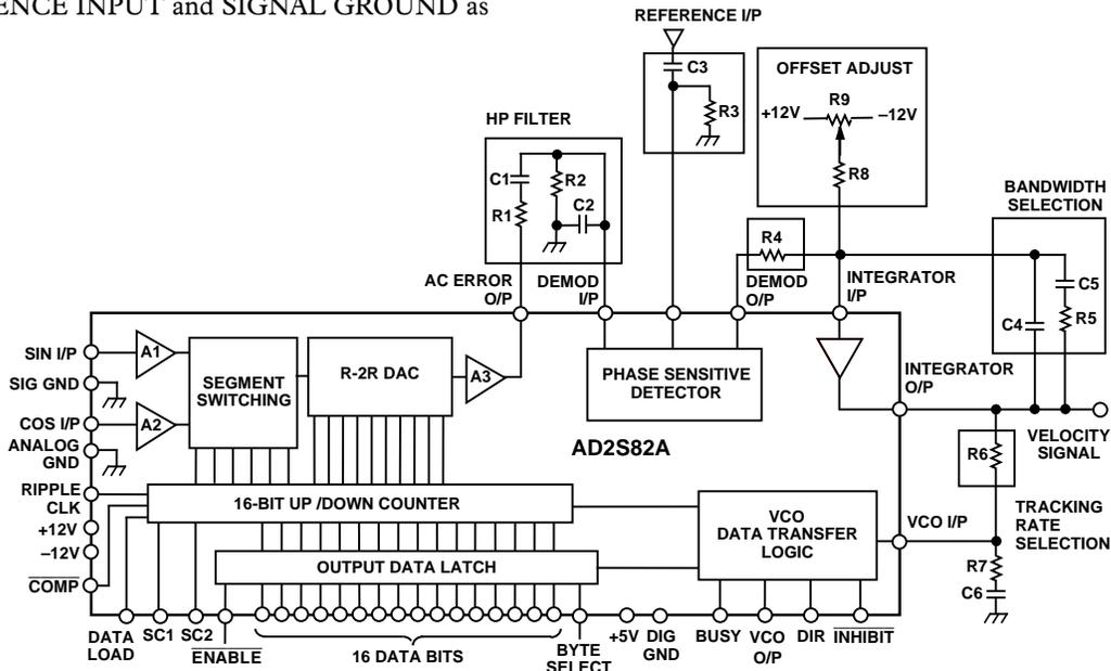
Figure 1a. AD2S82A Connection Diagram
