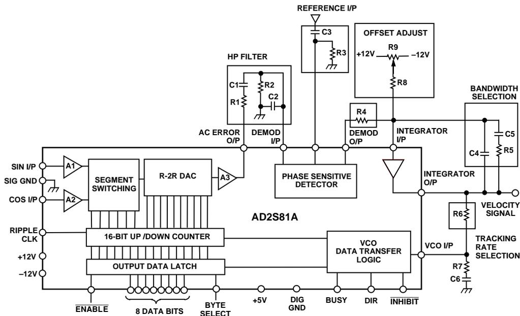
Figure 1b. AD2S81A Connection Diagram
