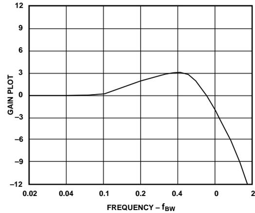
Figure 5. AD2S81A/AD2S82A Gain Plot
