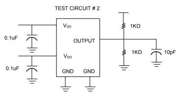
For parameter  $t_8$  (output skew rate) on -1H devices
