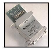
This RS-232 to RS-422 converter converts unbalanced RS-232 signals to balanced RS-422 signals. The power used for this converter is derived from the transmit data line (pin 2) and the handshake control lines (pins 4, 5, 6, 8, and 20). The converter can derive power from these lines
