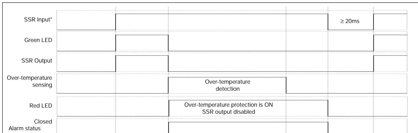
\*After over-temperature condition is removed, SSR can be reset by switching OFF the control input for more than 20 ms and switching back ON: this will switch ON the SSR output
