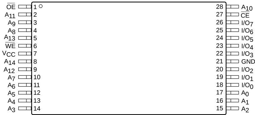
TSOP Top View (8mm X 13.4mm) (T13)
