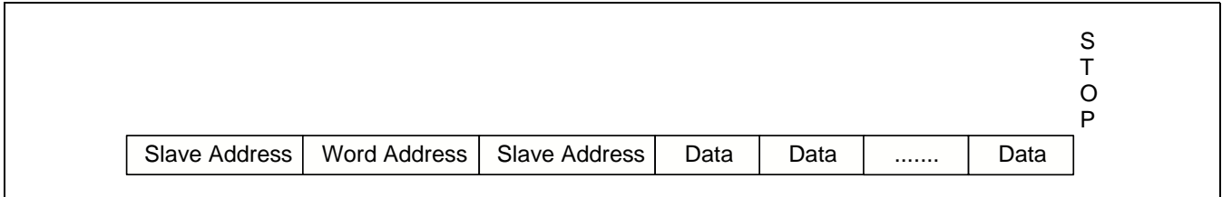
Figure 40. Serial Byte Access- Sequential Read
