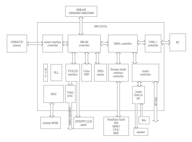
**Sensor Interface:** The sensor interface connects to the CMOS or CCD sensors. It can also connect to a video decoder to capture video. The SPCA533A has built-in a timing generator for the commonly used CCD sensors. A serial interface is used to program the CMOS sensors and external CDS/AGC chips for CCD sensors.
