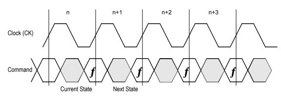
Current State and Next State Definition for: Pipeline and Flow through Read Write Control State Diagram
