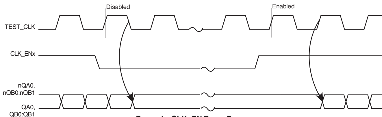
FIGURE 1. CLK_EN TIMING DIAGRAM
