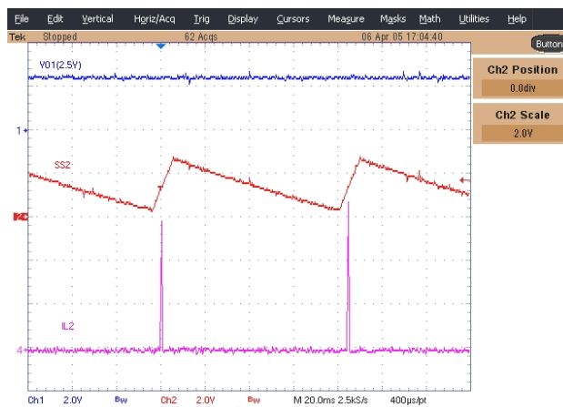
Figure 30 - 1.8V output shorted Ch1: Vo1, Ch2: SS2, Ch3: Inductor Current
