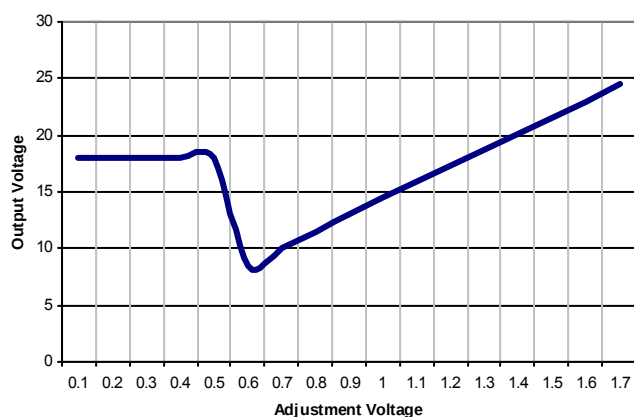
Figure 9 – Typical V_{OUT} versus V_{ADJ}
