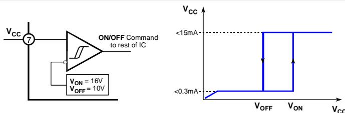
During Under-Voltage Lock-Out, the output driver is biased to a high impedance state. Pin 6 should be shunted to ground with a bleeder resistor to prevent activating the power switch with output leakage current.
