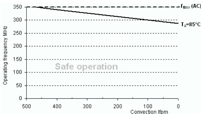
Figure 10. Maximum MPC9448 frequency, V_{CC} = 3.3V , MTBF 4 years, 4 pF load per line, 2s2p board
