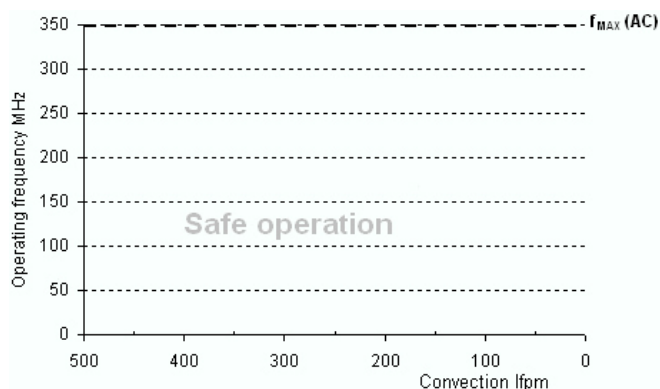
Figure 9. No maximum frequency limitation for V_{CC} = 3.3V , MTBF 4 years, driving series terminated transmission lines, 2s2p board
