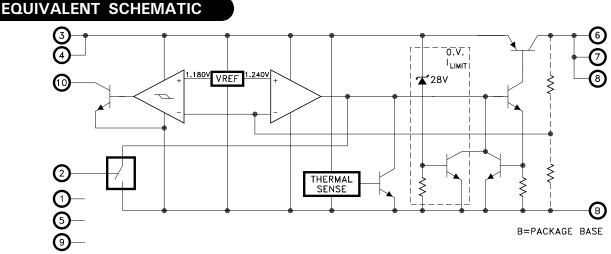
Schematic shown for fixed output voltage versions
