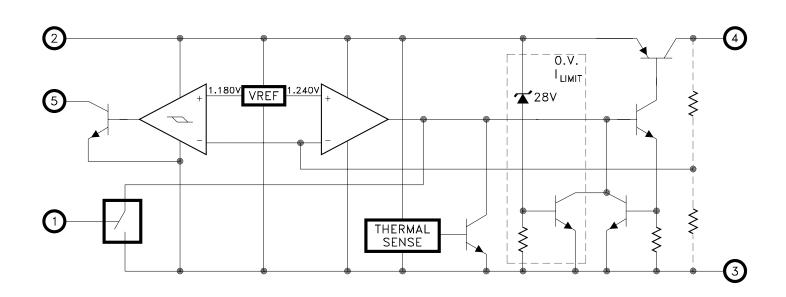
Schematic shown for fixed output voltage versions
