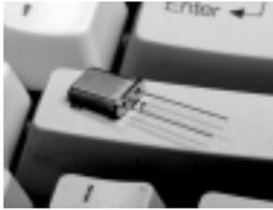
The UM series of miniature resistance weld crystals are suitable for applications where tight specs, small footprint, and wide frequency range is important.
