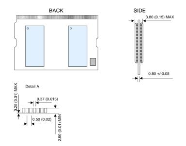
Note: All dimensions are typical with tolerances of +/- 0.15 unless otherwise stated. Units: Millimeters (Inches)
