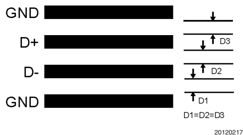
FIGURE 4. Ideal Diode Trace Layout
