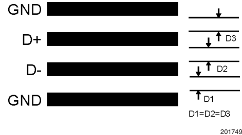
FIGURE 8. Ideal Diode Trace Layout
