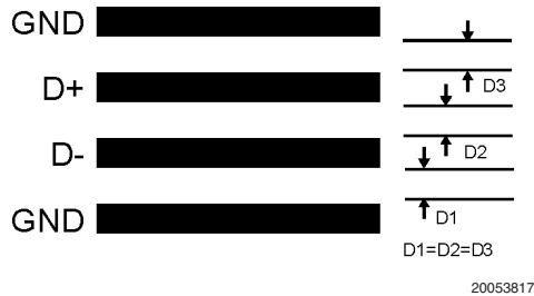
FIGURE 11. Ideal Diode Trace Layout
