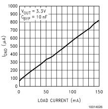
**Typical Performance Characteristics** Unless otherwise specified:  $C_{IN} = 1\mu$ F,  $C_{OUT} = 4.7\mu$ F,  $V_{IN} = V_{OUT}(NOM) + 1$ ,  $T_A = 25^{\circ}$ C, ON/OFF pin is tied to  $V_{IN}$ . (Continued)
