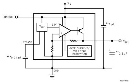
\*ON/OFF input must be actively terminated. Tie to V<sub>IN</sub> if this function is not to be used.
