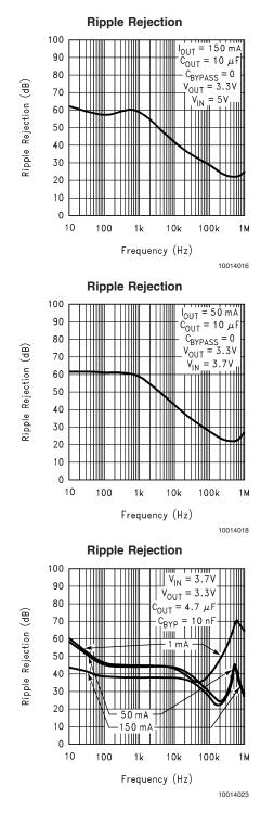
**Typical Performance Characteristics** Unless otherwise specified:  $C_{IN} = 1\mu$ F,  $C_{OUT} = 4.7\mu$ F,  $V_{IN} = V_{OUT}(NOM) + 1$ ,  $T_A = 25^{\circ}$ C, ON/OFF pin is tied to  $V_{IN}$ . (Continued)
