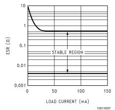
**Important:** The output capacitor must maintain its ESR within the stable region over the full operating temperature range of the application to assure stability.
