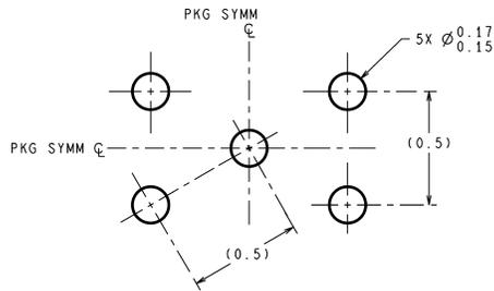
DIMENSIONS ARE IN MILLIMETERS
