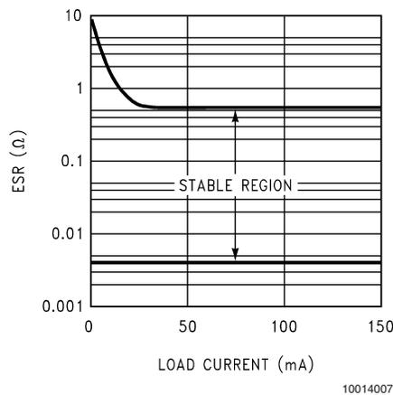
**Important:** The output capacitor must maintain its ESR within the stable region over the full operating temperature range of the application to assure stability.
