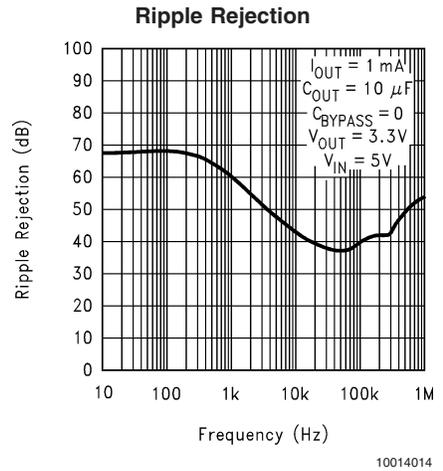
**Typical Performance Characteristics** Unless otherwise specified:  $C_{IN} = 1\mu F$ ,  $C_{OUT} = 4.7\mu F$ ,  $V_{IN} = V_{OUT(NOM)} + 1$ ,  $T_A = 25^\circ C$ , ON/OFF pin is tied to  $V_{IN}$ . (Continued)
