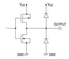
Schematic Diagram of Driver Output Circuit
