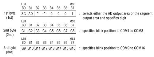
The 2nd and 3rd bytes (COM1 to COM16 position specification) are regarded as one data item, so 300 ns is sufficient for t<sub>DOFF</sub> time between bytes.
