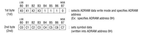
To specify symbol data continuously to the next address, specify only symbol data as follows. The address of ADRAM is automatically incremented. Specification of addresses is therefore unnecessary.
