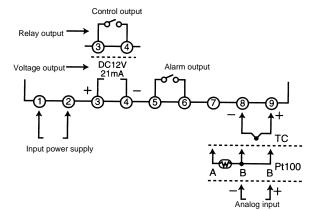
Standard insulation is applied to the power supply I/O sections. If reinforced insulation is required, connect the input and output terminals to a device without any exposed current-carrying parts or to a device with standard insulation suitable for the maximum operating voltage of the power supply I/O section.
