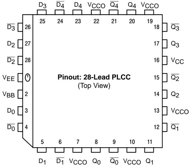
\* All VCC and VCCO pins are tied together on the die.
