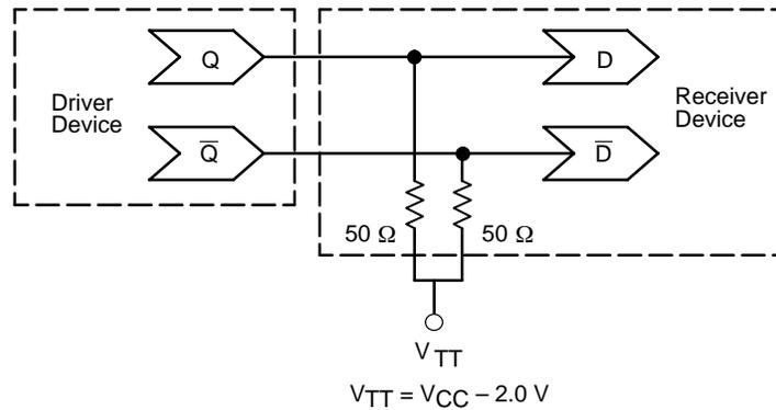
**Figure 1. Typical Termination for Output Driver and Device Evaluation**
