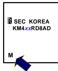
b. Top marking example of mirrored package
