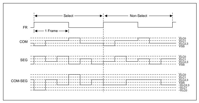
Figure 14-7. Select/No-Select Signal in 1/3 Duty, 1/3 Bias Display Mode
