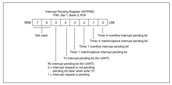
Figure 17-2. UART Interrupt Pending Bits (INTPND.5-.4)
