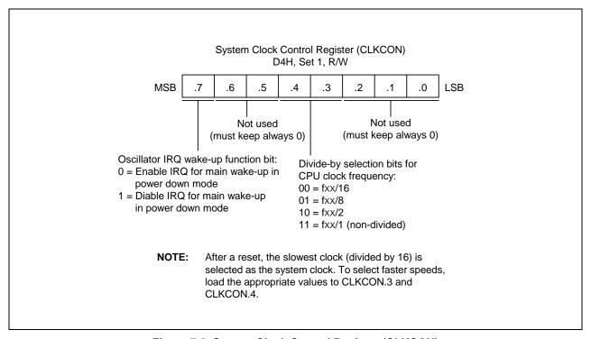
Figure 7-8. System Clock Control Register (CLKCON)
