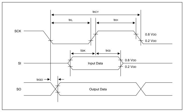
Figure 20-6. Serial Data Transfer Timing
