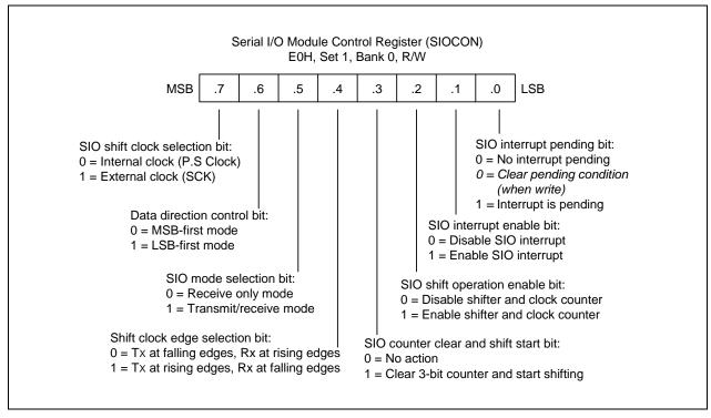
Figure 16-1. Serial I/O Module Control Registers (SIOCON)
