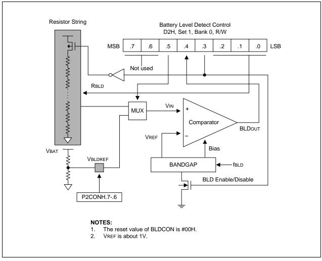
Figure 18-3. Battery Level Detector Circuit and Block Diagram
