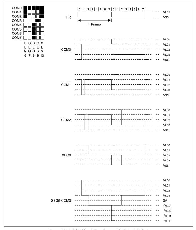
Figure 14-10. LCD Signal Waveforms (1/8 Duty, 1/4 Bias)
