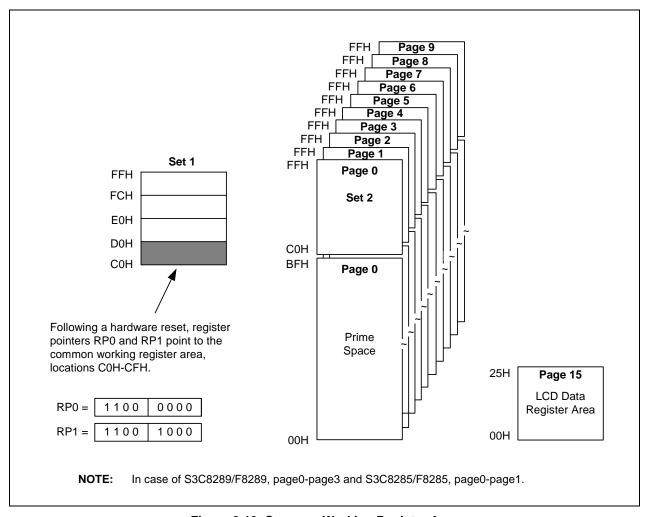
Figure 2-13. Common Working Register Area
