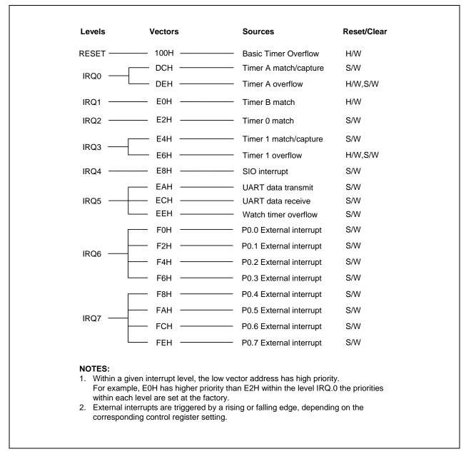
Figure 5-2. S3C828B/C8289/C8285 Interrupt Structure
