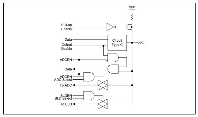
Figure 1-10. Pin Circuit Type F-2 (P2.7)
