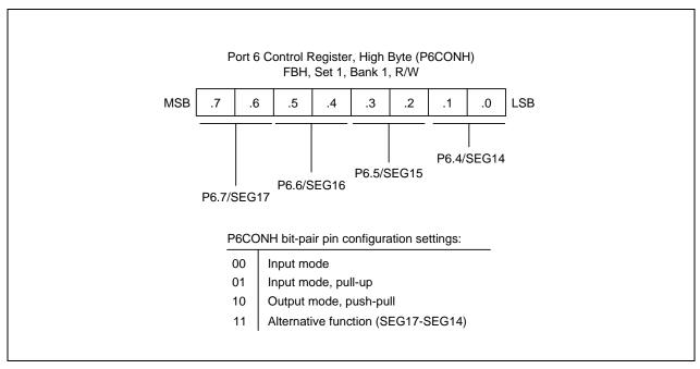
Figure 9-19. Port 6 High-byte Control Register (P6CONH)
