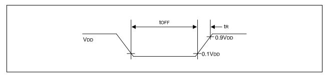
Figure 20-5. LVR (Low Voltage Reset) Timing
