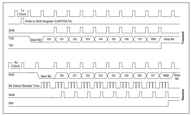
Figure 17-9. Timing Diagram for Serial Port Mode 3 Operation
