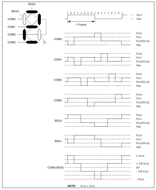
Figure 14-9. LCD Signal Waveforms (1/4 Duty, 1/3 Bias)
