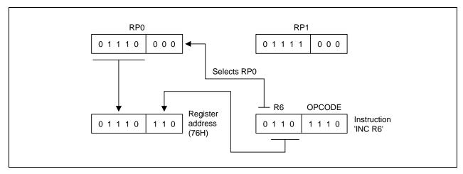
Figure 2-15. 4-Bit Working Register Addressing Example
