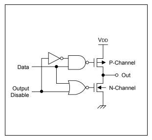
Figure 1-6. Pin Circuit Type C
