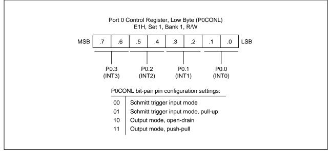
Figure 9-2. Port 0 Low-Byte Control Register (P0CONL)
