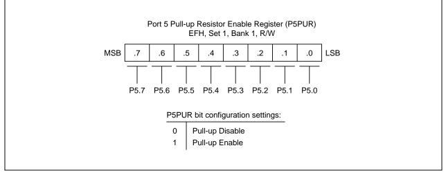
Figure 9-18. Port 5 Pull-up Resistor Enable Register (P5PUR)
