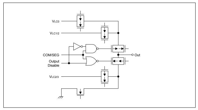
Figure 1-11. Pin Circuit Type H-4
