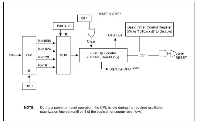
Figure 10-2. Basic Timer Block Diagram
