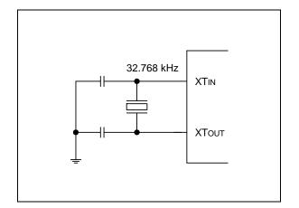
Figure 7-4. Crystal Oscillator (fxt, Normal)
