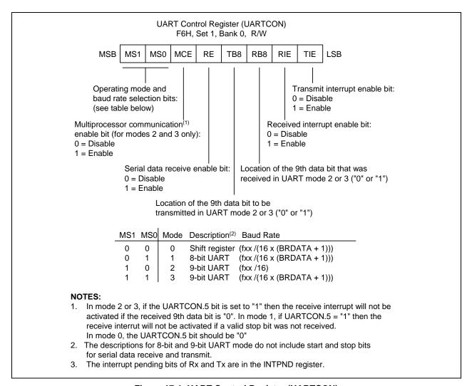
Figure 17-1. UART Control Register (UARTCON)
