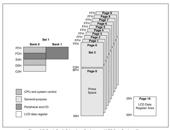
Figure 2-7. Set 1, Set 2, Prime Area Register, and LCD Data Register Map
