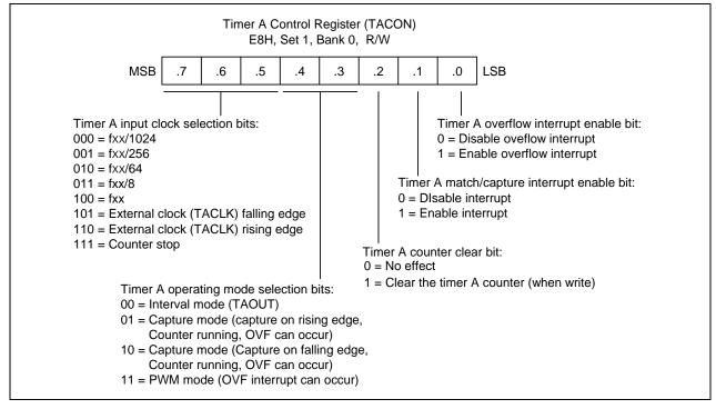
Figure 11-1. Timer A Control Register (TACON)
