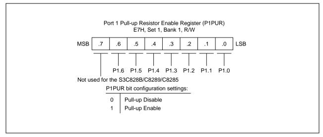
Figure 9-8. Port 1 Pull-up Resistor Enable Register (P1PUR)
