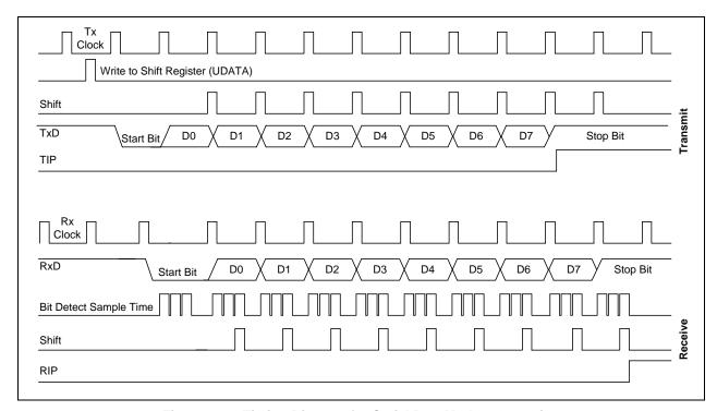
Figure 17-7. Timing Diagram for Serial Port Mode 1 Operation
