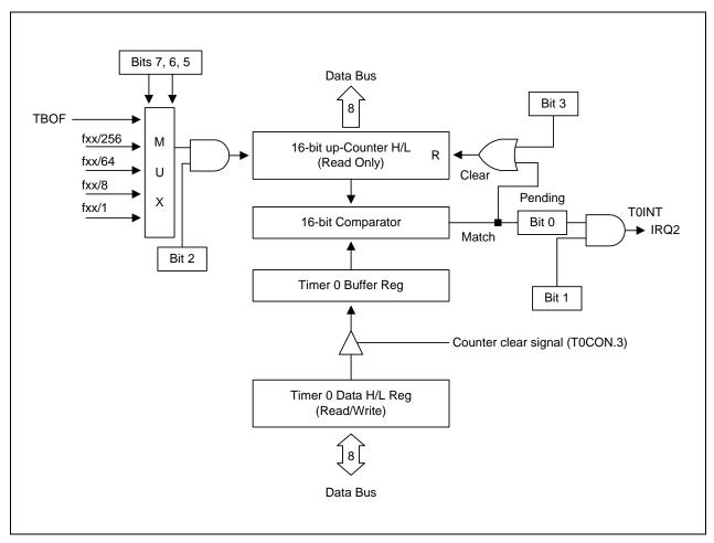
Figure 12-2. Timer 0 Functional Block Diagram
