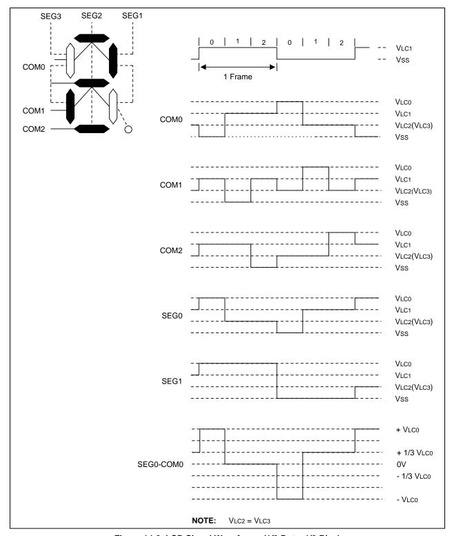
Figure 14-8. LCD Signal Waveforms (1/3 Duty, 1/3 Bias)
