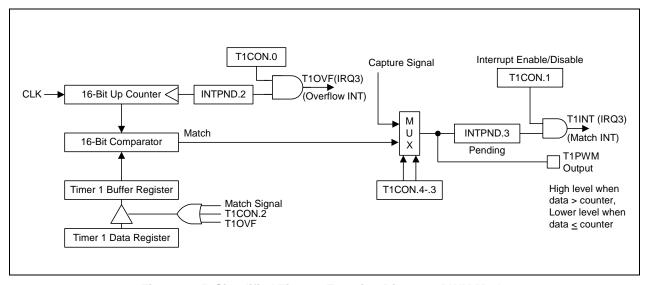
Figure 12-5. Simplified Timer 1 Function Diagram: PWM Mode
