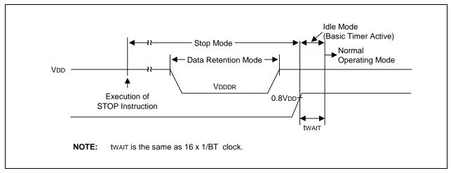
Figure 20-4. Stop Mode Release Timing Initiated by Interrupts
