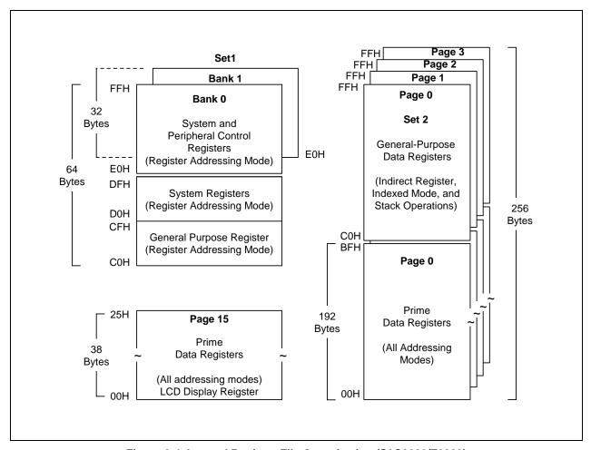
Figure 2-4. Internal Register File Organization (S3C8289/F8289)
