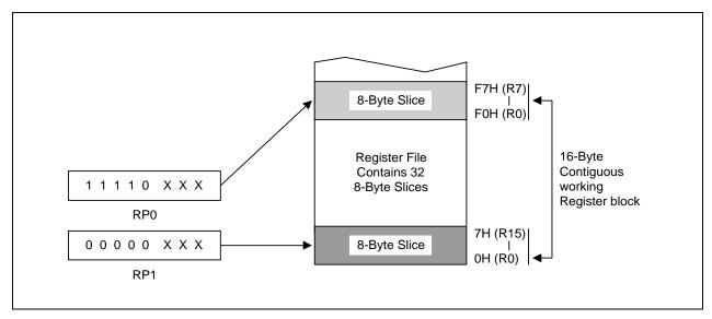
Figure 2-10. Non-Contiguous 16-Byte Working Register Block
