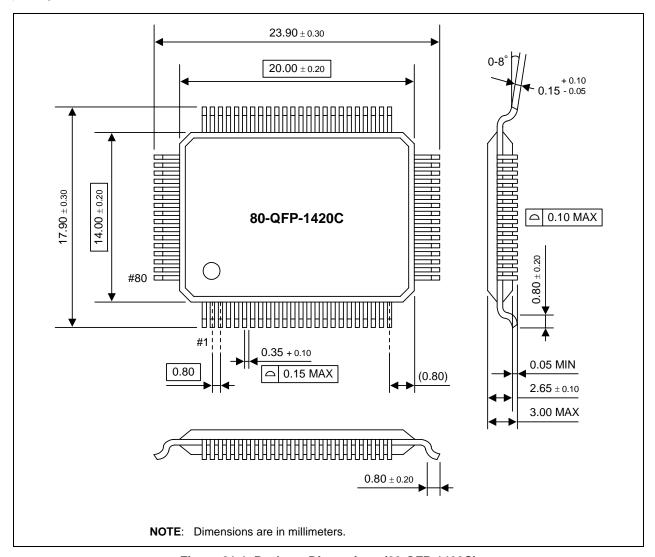
Figure 21-1. Package Dimensions (80-QFP-1420C)
