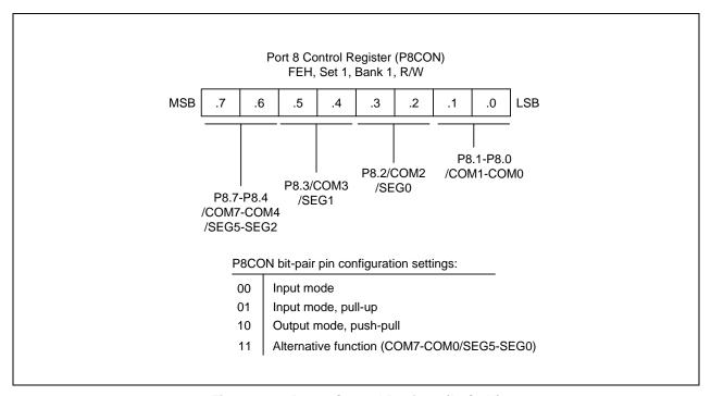
Figure 9-22. Port 8 Control Register (P8CON)
