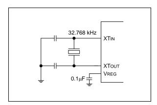
Figure 7-5. Crystal Oscillator (fxt, for Low Current)
