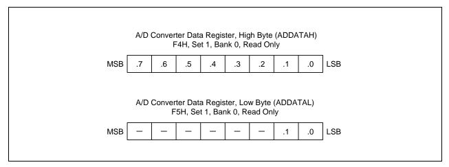
Figure 15-2. A/D Converter Data Register (ADDATAH/L)
