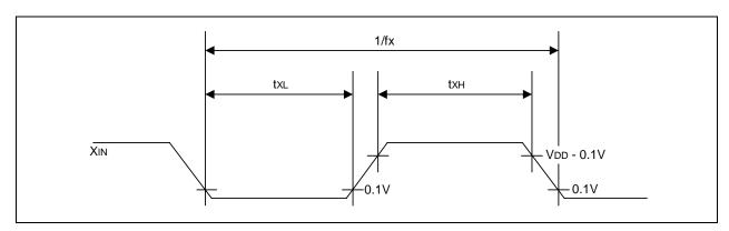
Figure 20-9. Clock Timing Measurement at  $\mathbf{X}_{\text{IN}}$
