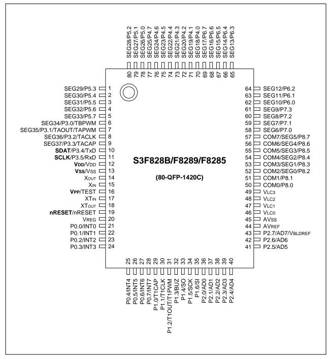
Figure 22-1. S3F828B/F8289/F8285 Pin Assignments (80-QFP-1420C)
