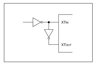
Figure 7-6. External Oscillator (fxT)
