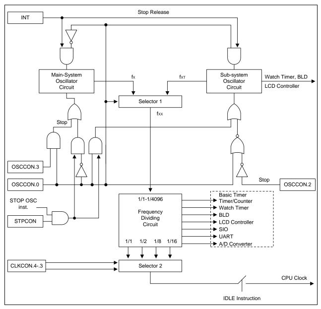
Figure 7-7. System Clock Circuit Diagram
