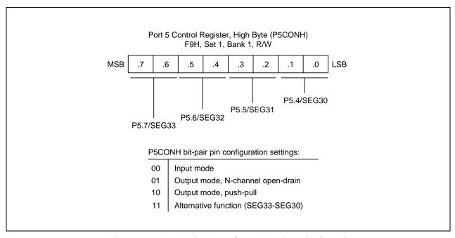
Figure 9-16. Port 5 High-Byte Control Register (P5CONH)
