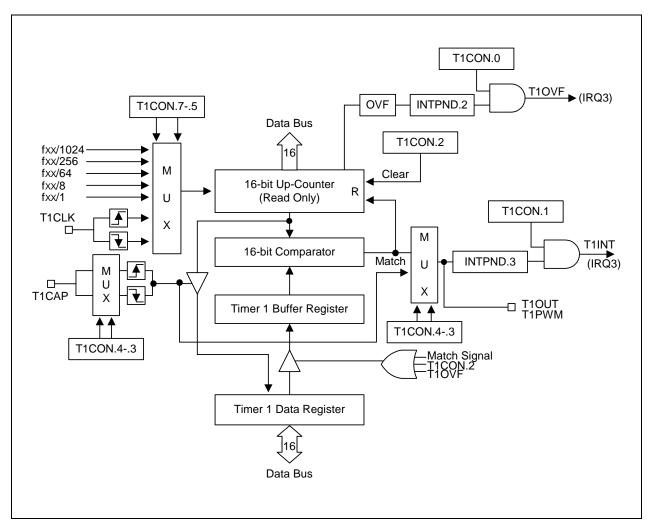
Figure 12-7. Timer 1 Functional Block Diagram
