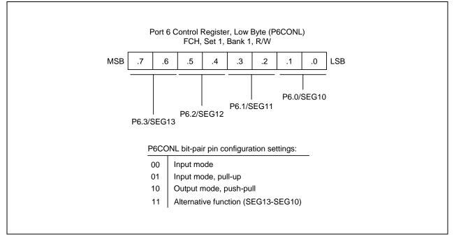
Figure 9-20. Port 6 Low-byte Control Register (P6CONL)
