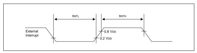
Figure 20-1. Input Timing for External Interrupts
