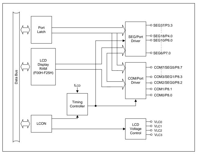
Figure 14-2. LCD Circuit Diagram
