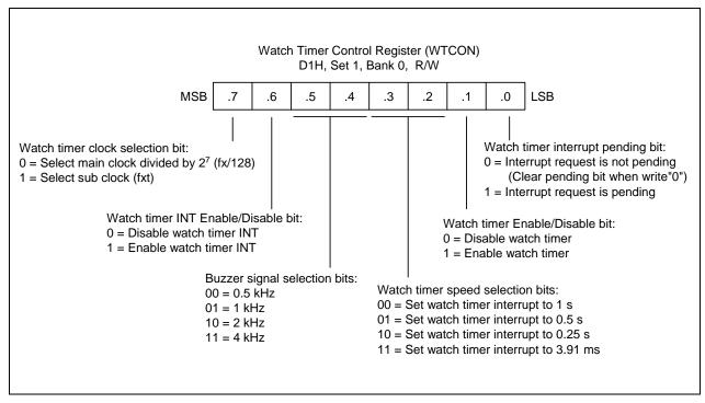
Figure 13-1. Watch Timer Control Register (WTCON)
