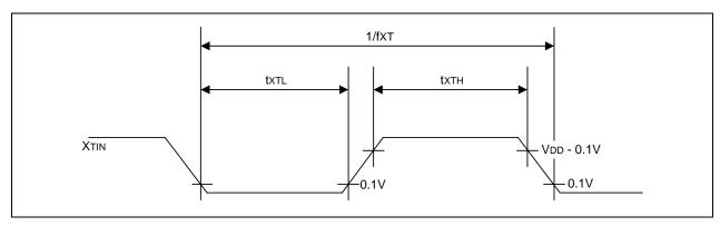
Figure 20-10. Clock Timing Measurement at  $\mathrm{XT}_{\mathrm{IN}}$
