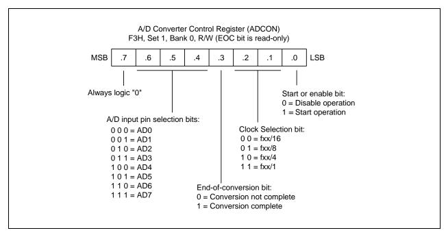
Figure 15-1. A/D Converter Control Register (ADCON)
