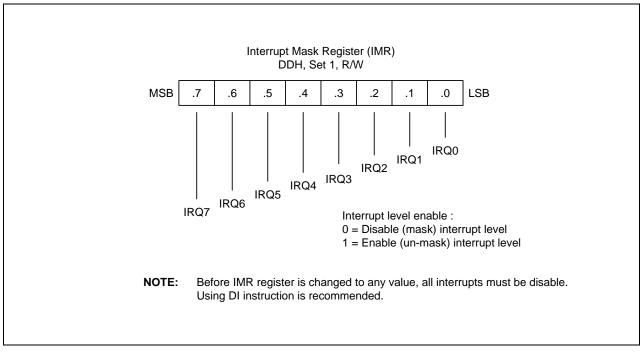
Figure 5-6. Interrupt Mask Register (IMR)
