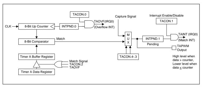
Figure 11-3. Simplified Timer A Function Diagram: PWM Mode
