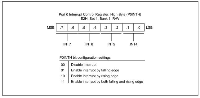
Figure 9-3. Port 0 High-Byte Interrupt Control Register (P0INTH)
