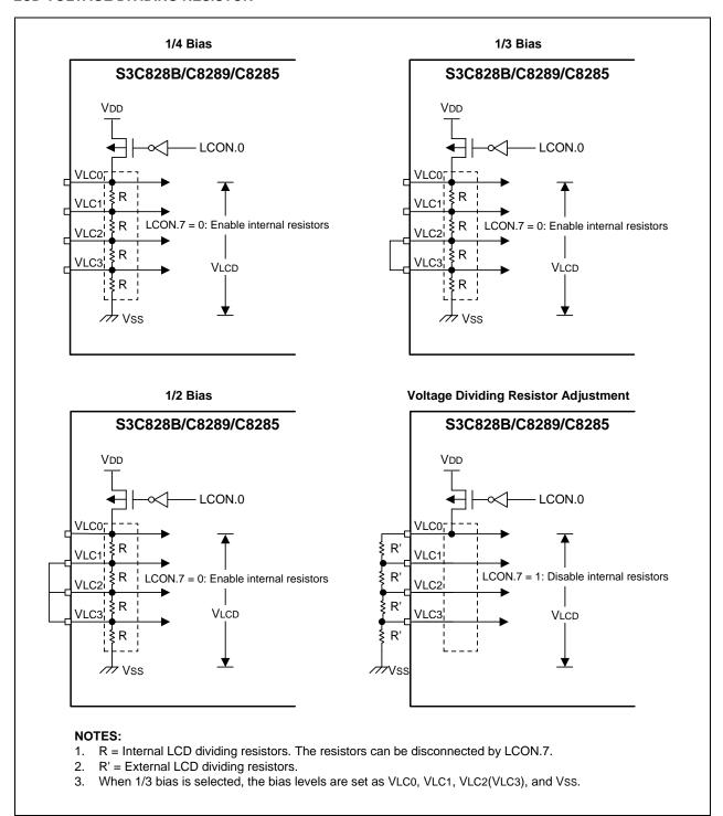
Figure 14-5. LCD Voltage Dividing Resistor Connection
