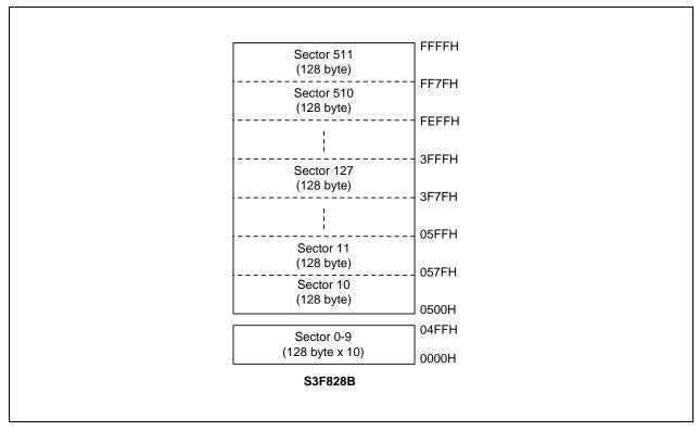
Figure 19-6. Sector Configurations in User Program Mode
