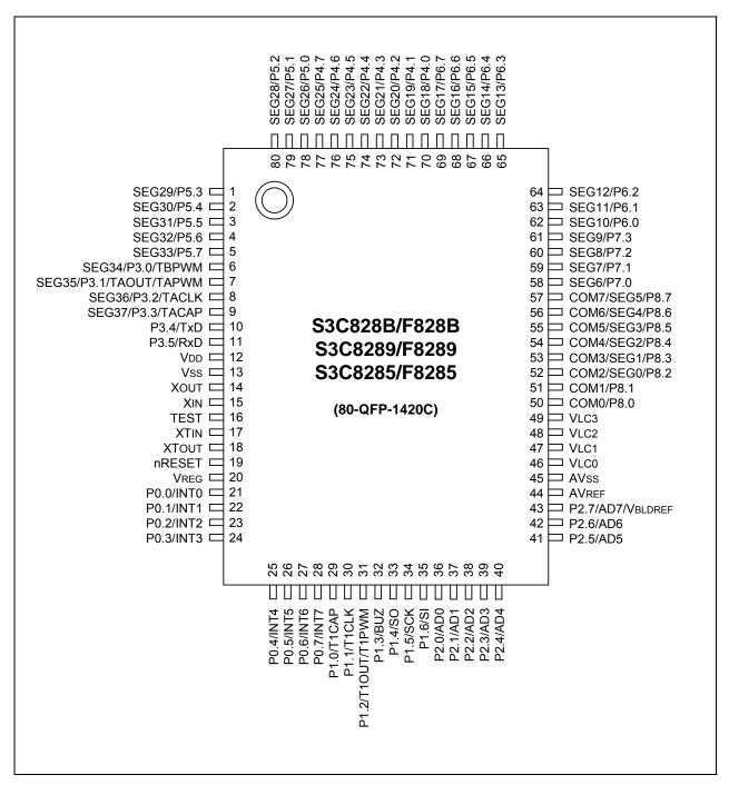
Figure 1-2. S3C828B/F828B/C8289/F8289/C8285/F8285 Pin Assignments (80-QFP-1420C)
