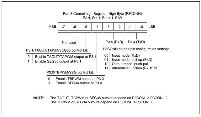
Figure 9-11. Port 3 High-Byte Control Register (P3CONH)
