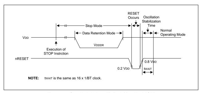
Figure 20-3. Stop Mode Release Timing Initiated by RESET
