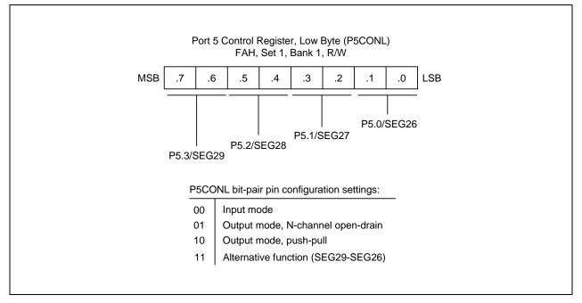
Figure 9-17. Port 5 Low-Byte Control Register (P5CONL)
