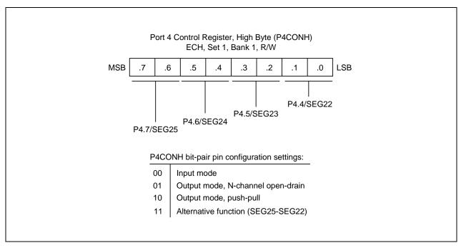
Figure 9-13. Port 4 High-Byte Control Register (P4CONH)
