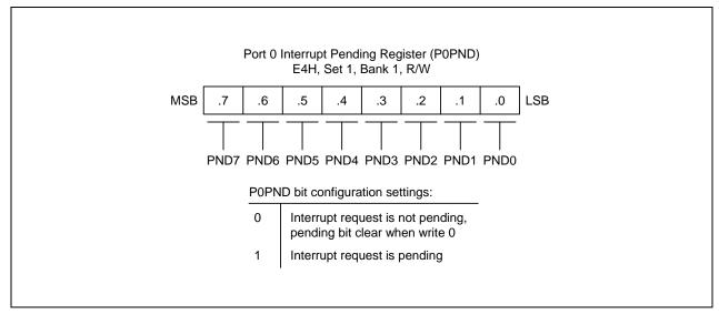
Figure 9-5. Port 0 Interrupt Pending Register (P0PND)
