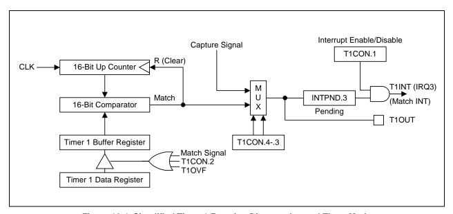
Figure 12-4. Simplified Timer 1 Function Diagram: Interval Timer Mode
