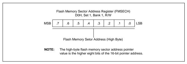
Figure 19-3. Flash Memory Sector Address Register High Byte (FMSECH)
