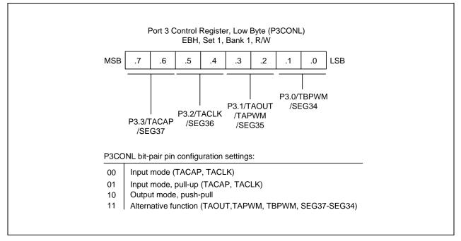
Figure 9-12. Port 3 Low-Byte Control Register (P3CONL)
