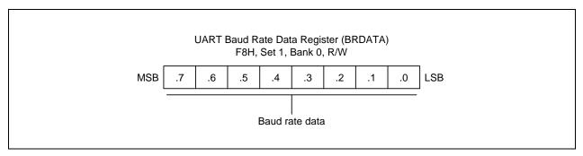
Figure 17-4. UART Baud Rate Data Register (BRDATA)
