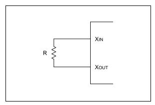
Figure 7-3. RC Oscillator (fx)
