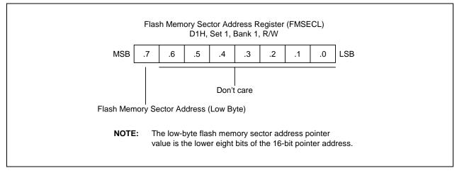
Figure 19-4. Flash Memory Sector Address Register Low Byte (FMSECL)
