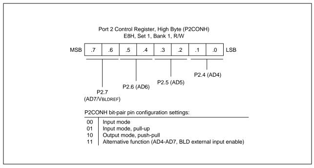
Figure 9-9. Port 2 High-Byte Control Register (P2CONH)
