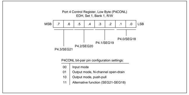
Figure 9-14. Port 4 Low-Byte Control Register (P4CONL)
