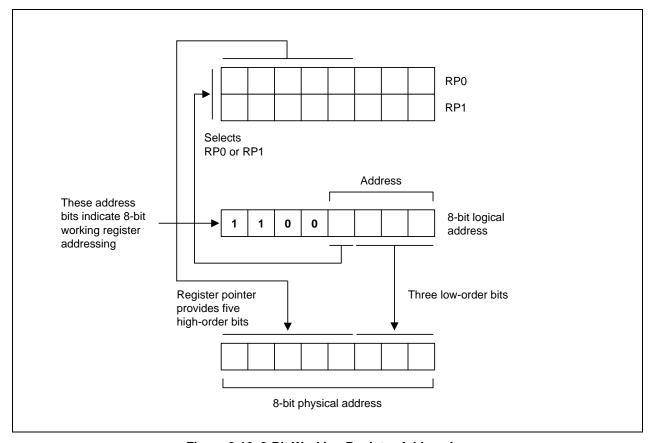
Figure 2-16. 8-Bit Working Register Addressing
