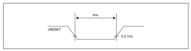
Figure 20-2. Input Timing for nRESET
