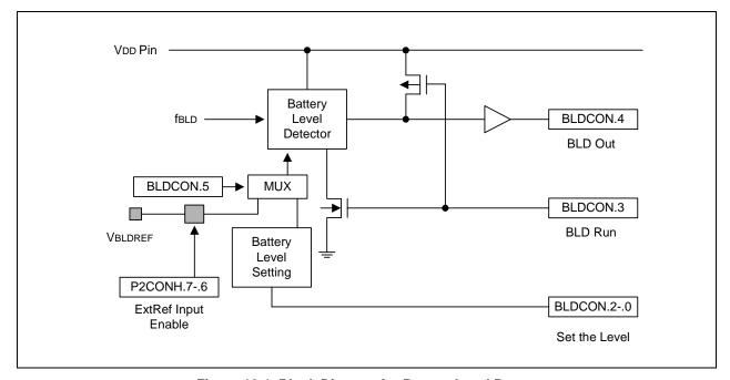
Figure 18-1. Block Diagram for Battery Level Detect
