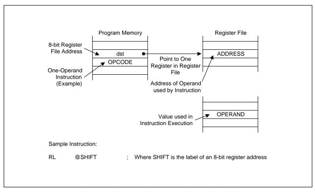
Figure 3-3. Indirect Register Addressing to Register File
