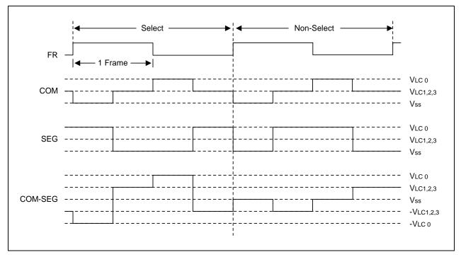
Figure 14-6. Select/No-Select Signal in 1/2 Duty, 1/2 Bias Display Mode
