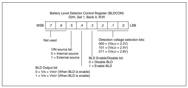
Figure 18-2. Battery Level Detector Control Register (BLDCON)
