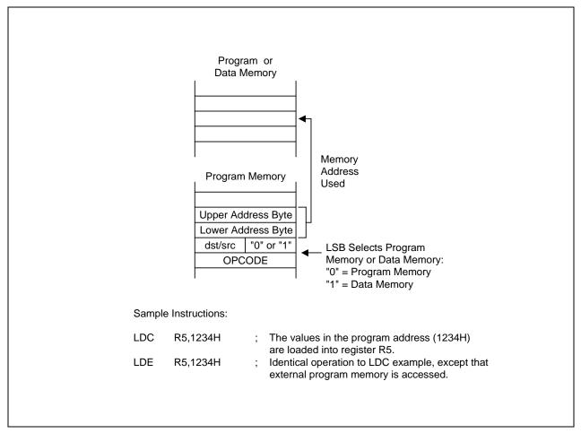
Figure 3-10. Direct Addressing for Load Instructions
