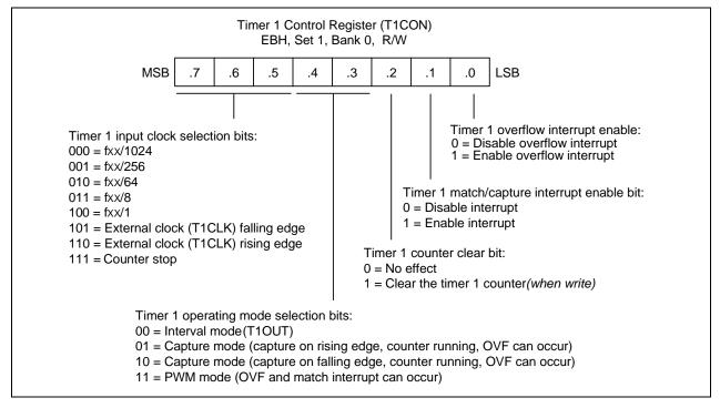
Figure 12-3. Timer 1 Control Register (T1CON)
