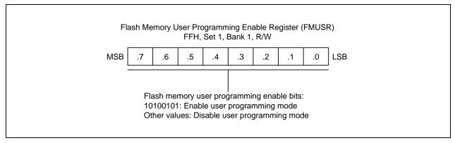
Figure 19-2. Flash Memory User Programming Enable Register (FMUSR)
