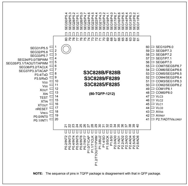
Figure 1-3. S3C828B/F828B/C8289/F8289/C8285/F8285 Pin Assignments (80-TQFP-1212)
