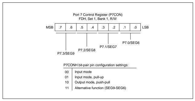
Figure 9-21. Port 7 Control Register (P7CON)
