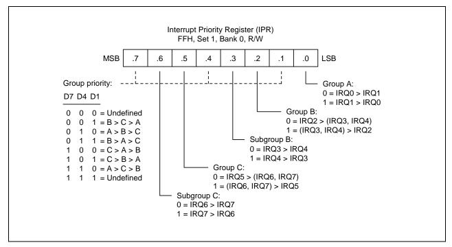
Figure 5-8. Interrupt Priority Register (IPR)
