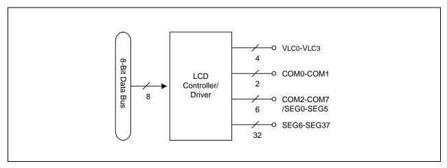
Figure 14-1. LCD Function Diagram
