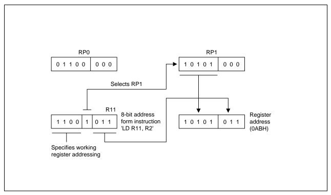
Figure 2-17. 8-Bit Working Register Addressing Example
