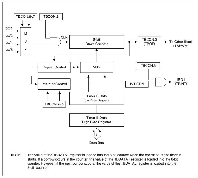
Figure 11-7. Timer B Functional Block Diagram
