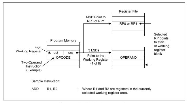
Figure 3-2. Working Register Addressing
