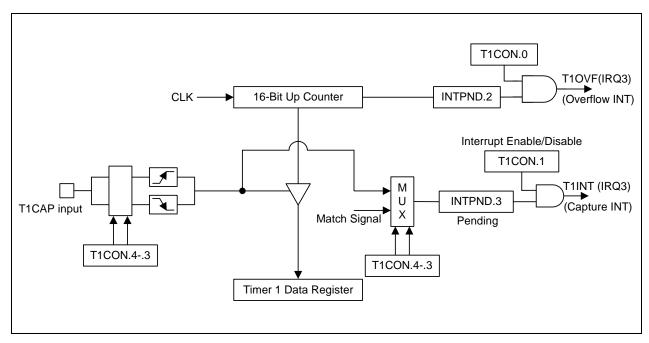
Figure 12-6. Simplified Timer 1 Function Diagram: Capture Mode
