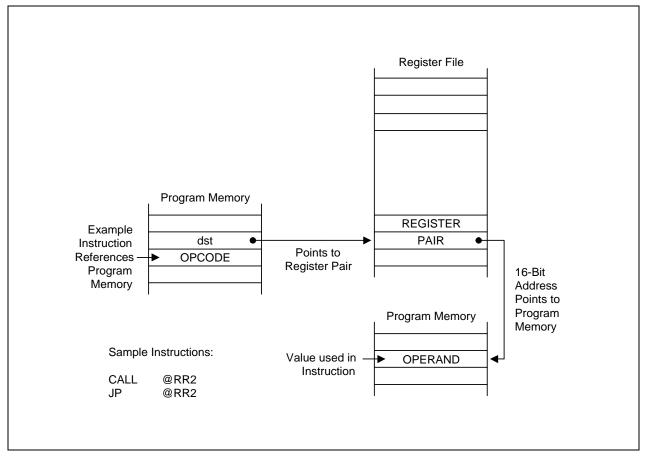
Figure 3-4. Indirect Register Addressing to Program Memory
