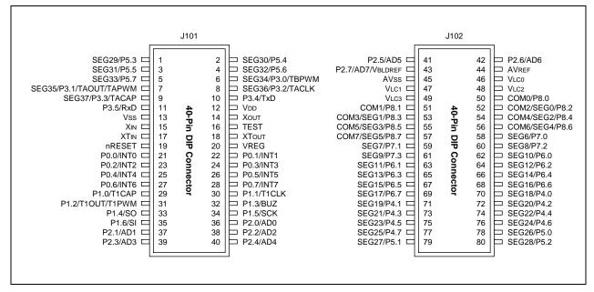
Figure 23-3. 40-Pin Connectors (J101, J102) for TB828B/9/5
