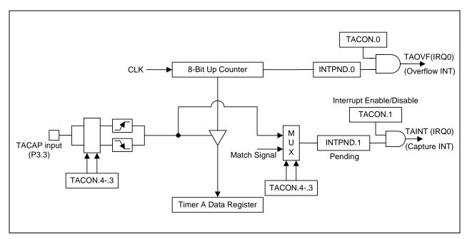
Figure 11-4. Simplified Timer A Function Diagram: Capture Mode
