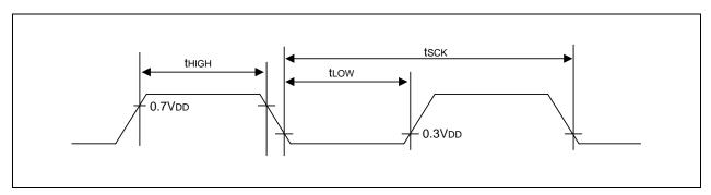
Figure 20-7. Waveform for UART Timing Characteristics
