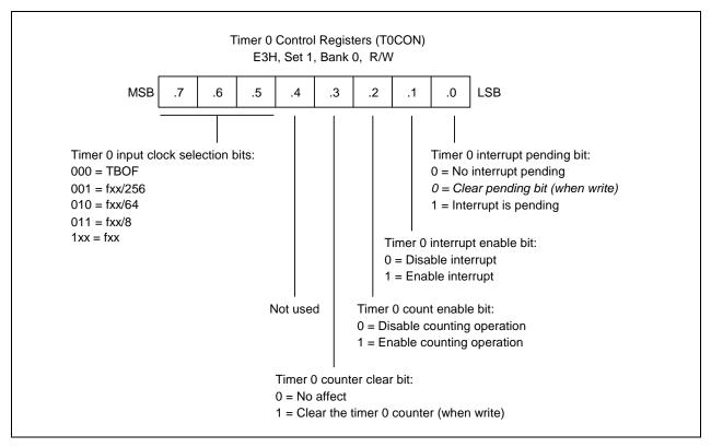
Figure 12-1. Timer 0 Control Register (T0CON)
