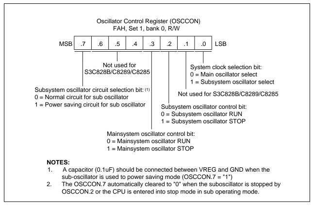
Figure 7-9. Oscillator Control Register (OSCCON)
