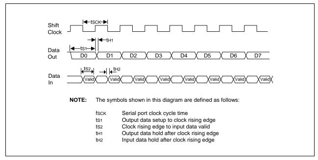
Figure 20-8. Timing Waveform for the UART Module
