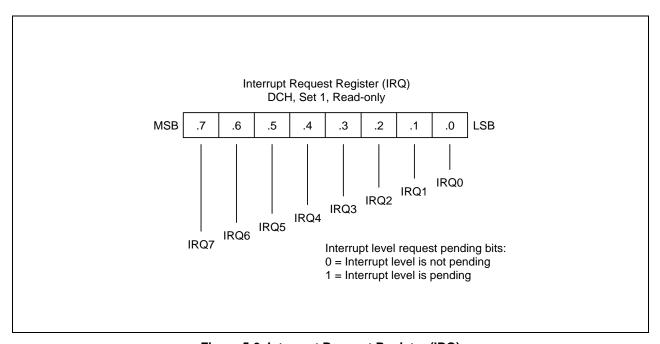
Figure 5-9. Interrupt Request Register (IRQ)
