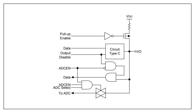
Figure 1-9. Pin Circuit Type F-1 (P2.0-P2.6)
