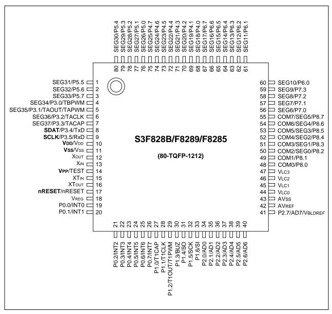
Figure 22-2. S3F828B/F8289/F8285 Pin Assignments (80-TQFP-1212)
