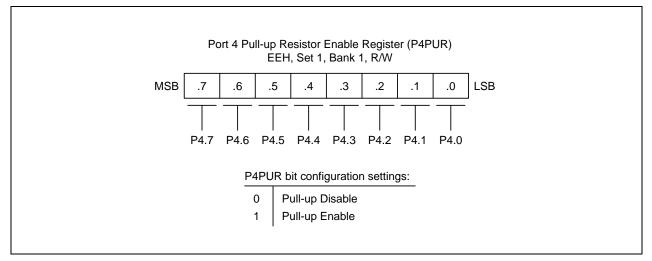
Figure 9-15. Port 4 Pull-up Resistor Enable Register (P4PUR)
