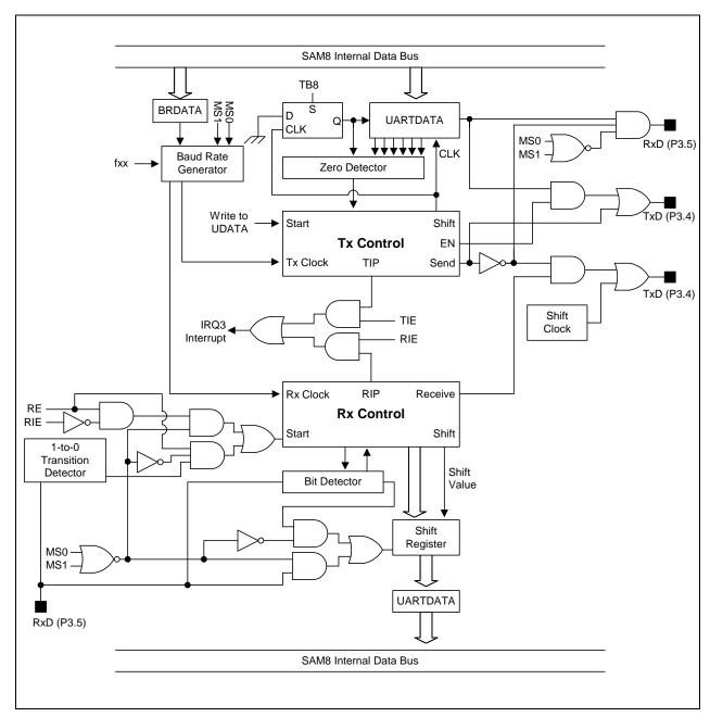
Figure 17-5. UART Functional Block Diagram
