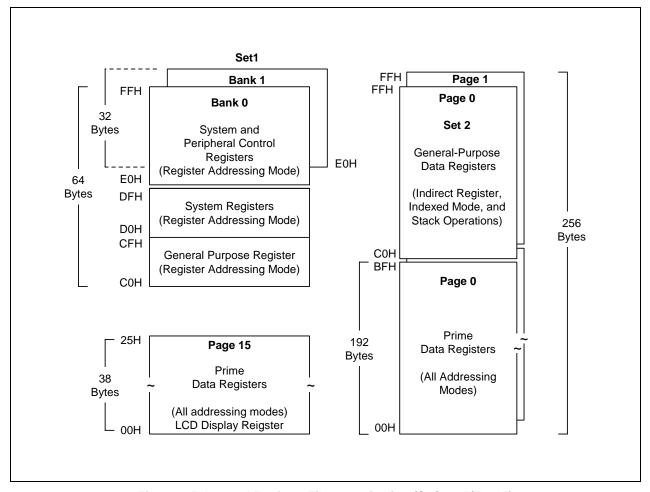
Figure 2-5. Internal Register File Organization (S3C8285/F8285)
