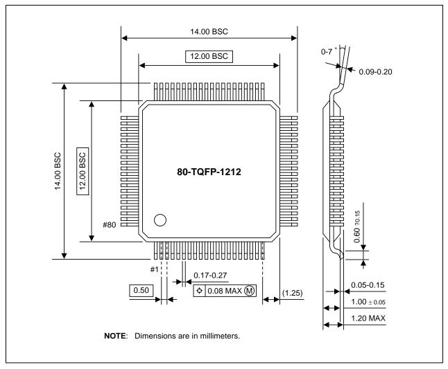
Figure 21-2. Package Dimensions (80-TQFP-1212)
