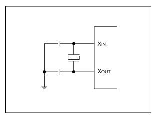
Figure 7-1. Crystal/Ceramic Oscillator (fx)
