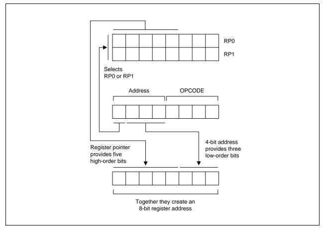
Figure 2-14. 4-Bit Working Register Addressing
