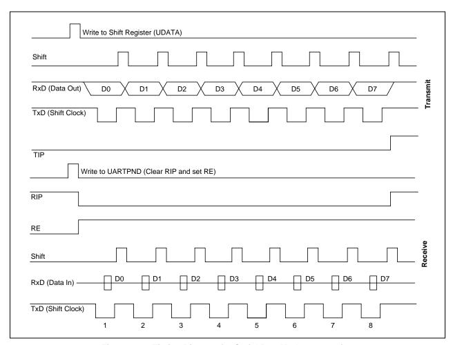
Figure 17-6. Timing Diagram for Serial Port Mode 0 Operation
