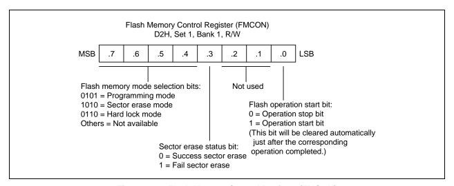
Figure 19-1. Flash Memory Control Register (FMCON)
