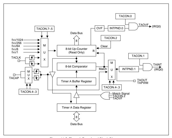
Figure 11-5. Timer A Functional Block Diagram
