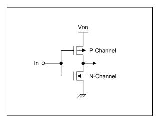
Figure 1-4. Pin Circuit Type A
