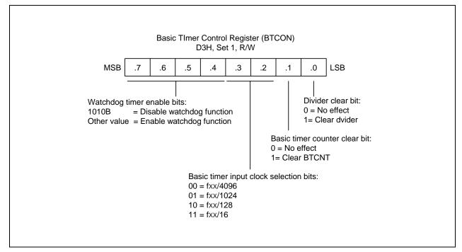
Figure 10-1. Basic Timer Control Register (BTCON)
