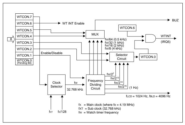
Figure 13-2. Watch Timer Circuit Diagram
