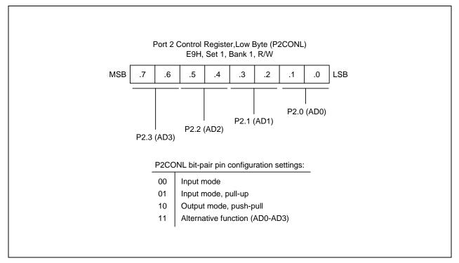
Figure 9-10. Port 2 Low-Byte Control Register (P2CONL)
