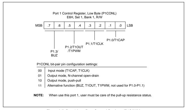
Figure 9-7. Port 1 Low-Byte Control Register (P1CONL)
