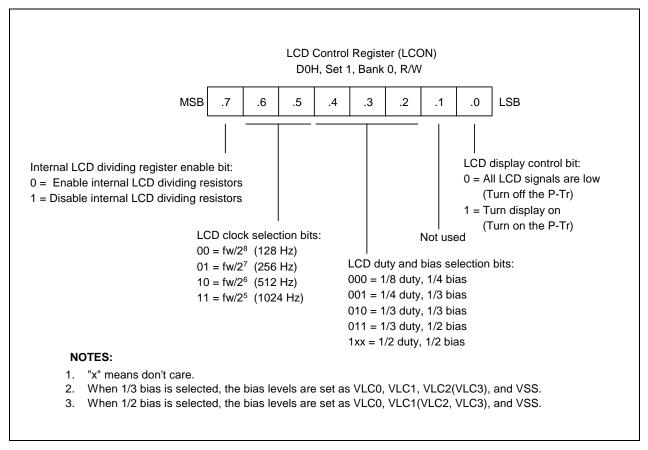
Figure 14-4. LCD Control Register (LCON)
