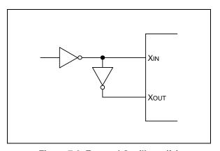
Figure 7-2. External Oscillator (fx)
