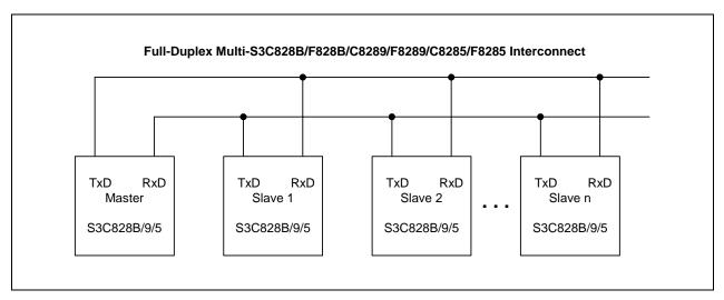
Figure 17-10. Connection Example for Multiprocessor Serial Data Communications
