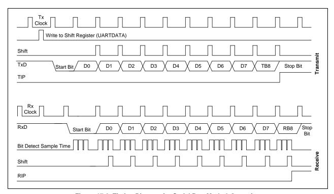
Figure 17-8. Timing Diagram for Serial Port Mode 2 Operation
