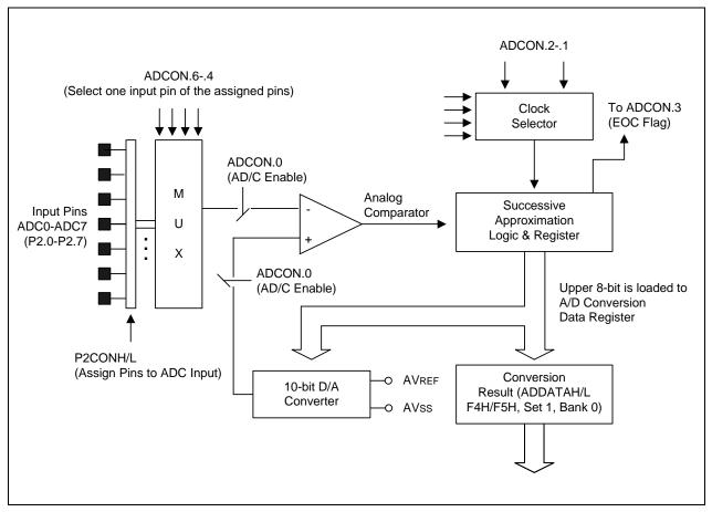
Figure 15-3. A/D Converter Functional Block Diagram
