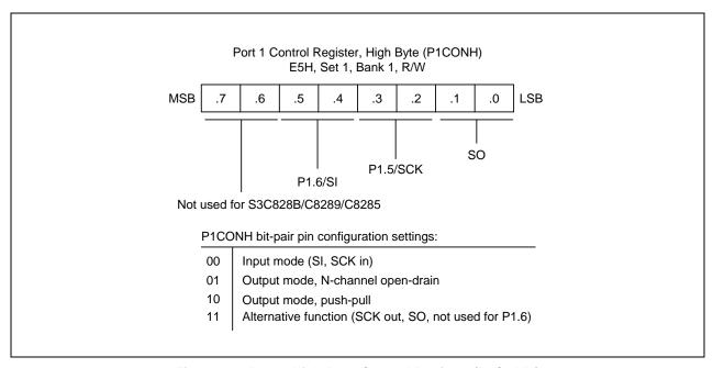
Figure 9-6. Port 1 High-Byte Control Register (P1CONH)
