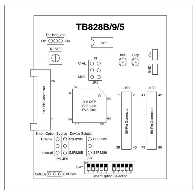
Figure 23-2. TB828B/9/5 Target Board Configuration
