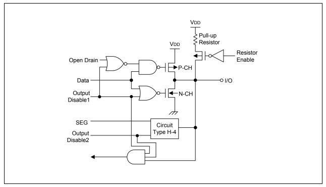
Figure 1-12. Pin Circuit Type H-8 (P4, P5)
