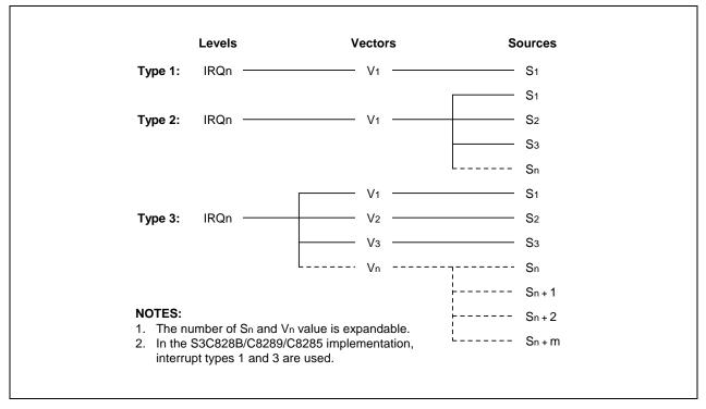
Figure 5-1. S3C8-Series Interrupt Types
