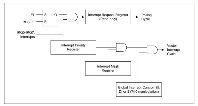
Figure 5-4. Interrupt Function Diagram
