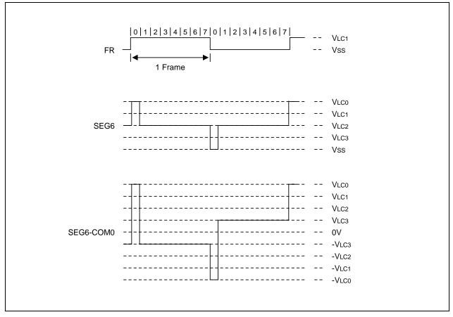
Figure 14-10. LCD Signal Waveforms (1/8 Duty, 1/4 Bias) (Continued)
