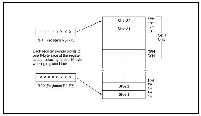
Figure 2-8. 8-Byte Working Register Areas (Slices)
