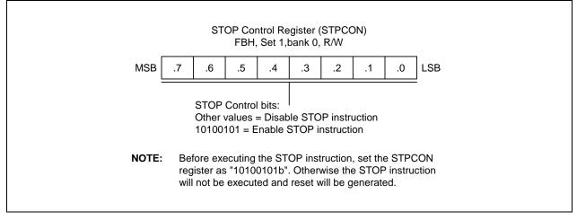
Figure 7-10. STOP Control Register (STPCON)
