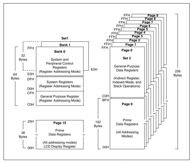
Figure 2-3. Internal Register File Organization (S3C828B/F828B)
