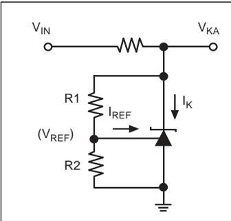
Figure 3. Test Circuit for  $V_{KA} > V_{REF}$
