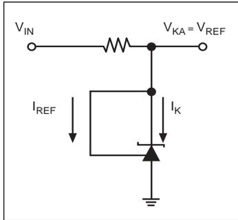
Figure 2. Test Circuit for  $V_{KA} = V_{REF}$
