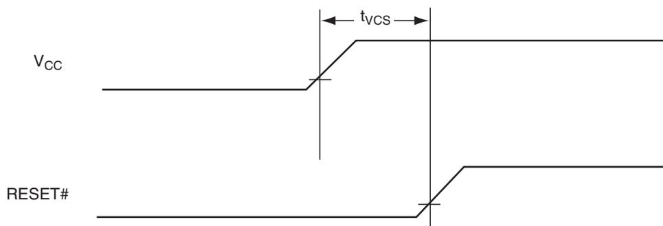
Figure I3. V<sub>CC</sub> Power-up Diagram
