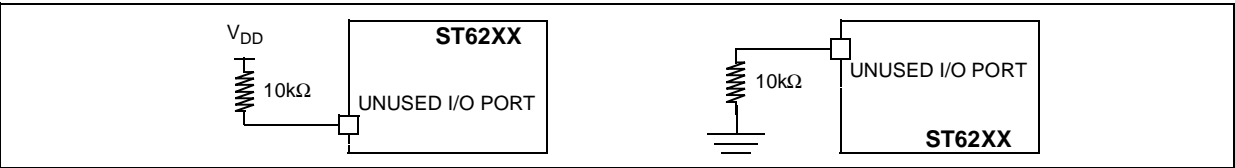
Figure 62. Two typical Applications with unused I/O Pin
