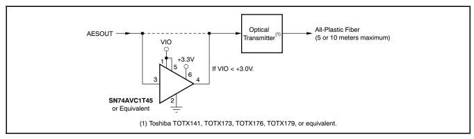
Figure 90. Interfacing to an Optical Transmitter Module
