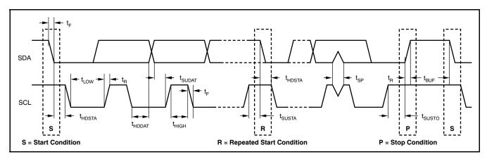
Figure 3. I<sup>2</sup>C Standard and Fast Mode Timing
