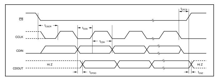
Figure 2. SPI Interface Timing
