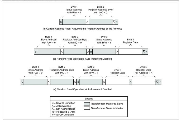
Figure 78. Fast/Standard Mode Read Operations
