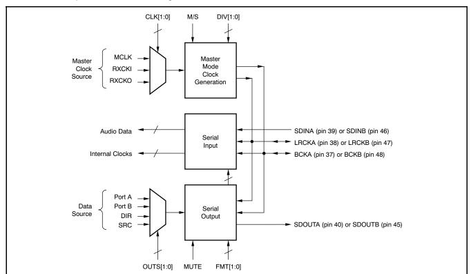
Figure 61. Audio Serial Port Block Diagram
