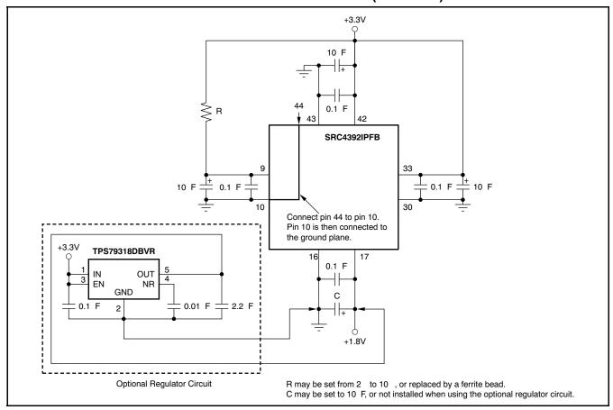
Figure 82. Recommended Power-Supply Connections
