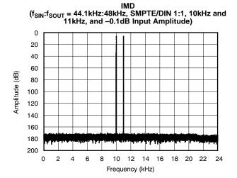
IMD (f<sub>SIN</sub>:f<sub>SOUT</sub> = 48kHz:44.1kHz, SMPTE/DIN 1:1, 10kHz and 11kHz, and -0.1dB Input Amplitude)
