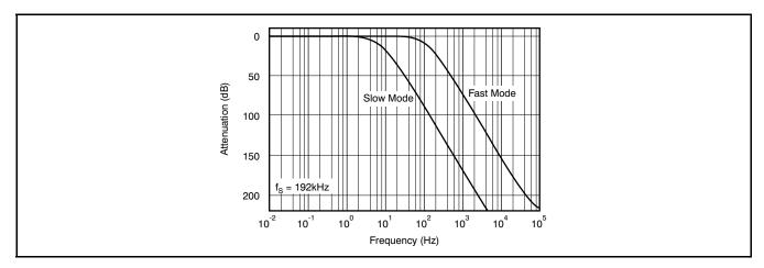
Figure 74. Output Digital Servo-Loop Frequency Response
