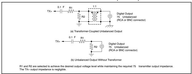
Figure 89. Unbalanced Line Output Interfaces
