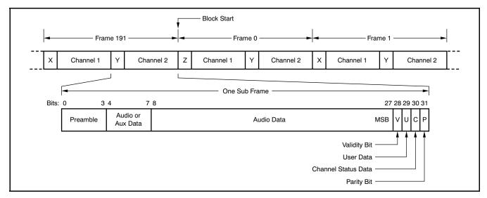
Figure 63. AES3 Frame and Subframe Encoding
