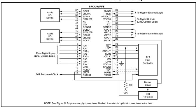
Figure 80. Typical Application Diagram Using SPI Host Interface
