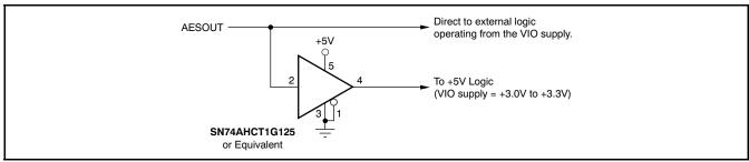
Figure 91. CMOS/TTL Output Logic Interface
