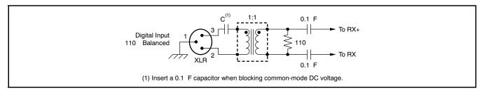
Figure 83. Transformer-Coupled Balanced Input Interface
