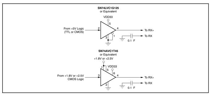
Figure 87. CMOS/TTL Input Logic Interface
