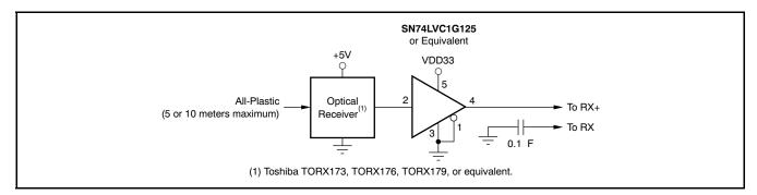
Figure 86. Interfacing to a +5V Optical Receiver Module
