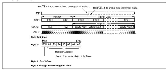
Figure 75. Serial Peripheral Interface (SPI) Protocol for the SRC4392
