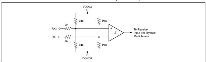
Figure 68. Differential Line Receiver Circuit
