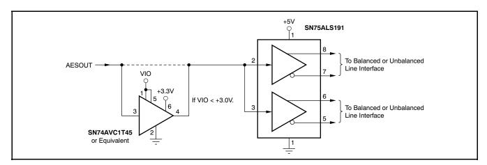
Figure 92. External Line Driver Interface
