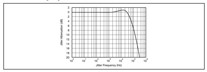
Figure 69. DIR Jitter Attenuation Characteristics
