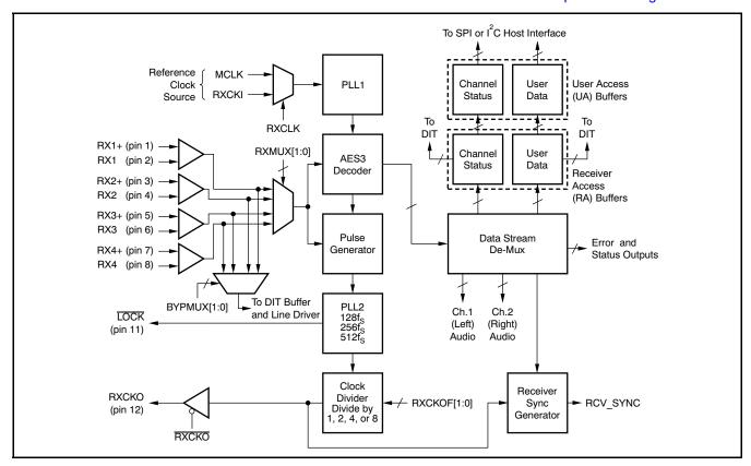
Figure 67. Digital Interface Receiver (DIR) Functional Block Diagram
