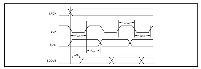
Figure 1. Audio Serial Port Timing
