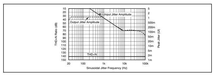
Figure 70. DIR Jitter Tolerance Plot
