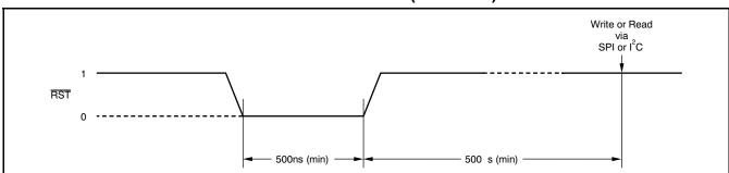
Figure 60. Reset Sequence Timing
