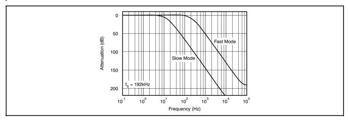
Figure 73. Input Digital Servo-Loop Frequency Response
