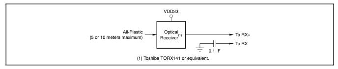
Figure 85. Interfacing to a +3.3V Optical Receiver Module
