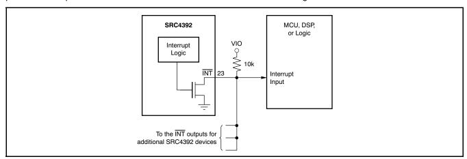
Figure 79. Interrupt Output Pin Connections
