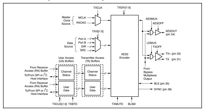
Figure 65. Digital Interface Transmitter (DIT) Functional Block Diagram
