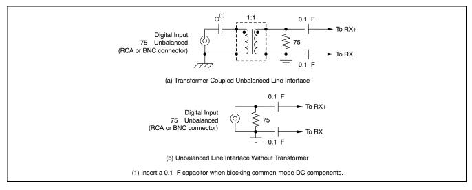
Figure 84. Unbalanced Line Input Interfaces
