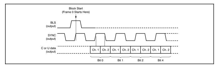
Figure 71. DIR Channel Status and User Data Serial Output Format Via the GPO Pins
