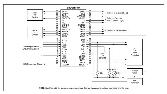
Figure 81. Typical Application Diagram Using I<sup>2</sup>C Host Interface
