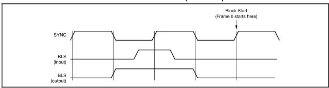
Figure 66. DIT Block Start Timing
