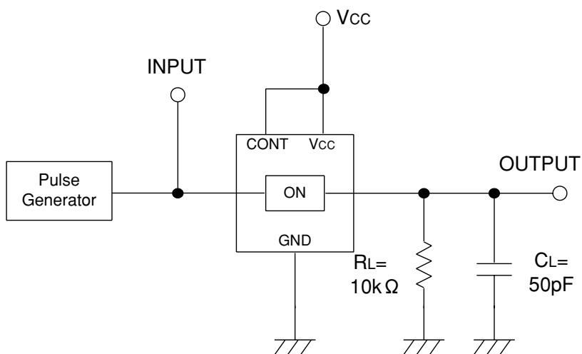
Note: Open output when measuring supply current
