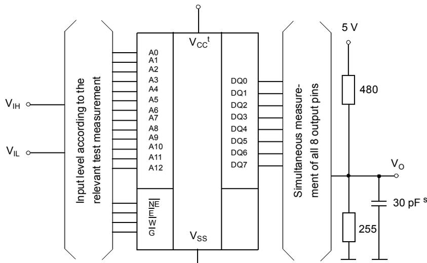
s: In measurement of  $t_{dis}$ -times and  $t_{en}$ -times the capacitance is 5 pF.
