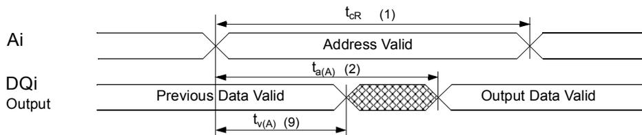
**Read Cycle 2:  $\bar{G}$ -,  $\bar{E}$ -controlled (during Read cycle:  $\bar{W} = \bar{NE} = V_{IH}$ )<sup>g</sup>**
