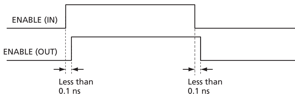
Figure 2-31 • Timing Diagram (Option 1: Bypasses Skew Circuit)
