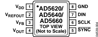
Figure 4. MSOP Pin Configuration
