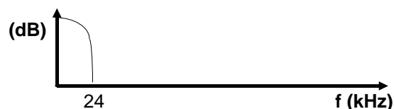
Figure 26. Spectrum After Continuous Time Filter
