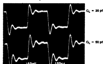
Pulse Response with V_+ = 3V, V_- = -2V
