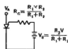
b) Equivalent Test Circuit
