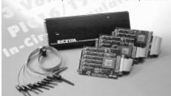
RICE17A with different processor modules and external probe cable
