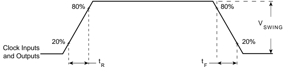
FIGURE 5 - INPUT AND OUTPUT RISE AND FALL TIME
