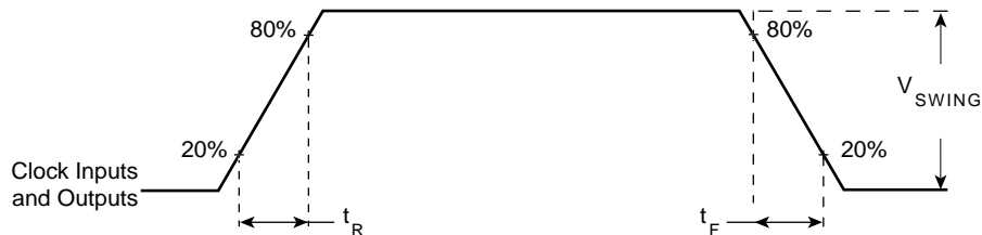
FIGURE 3 - INPUT AND OUTPUT RISE AND FALL TIME
