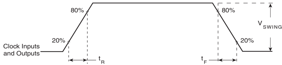
FIGURE 5 - INPUT AND OUTPUT RISE AND FALL TIME
