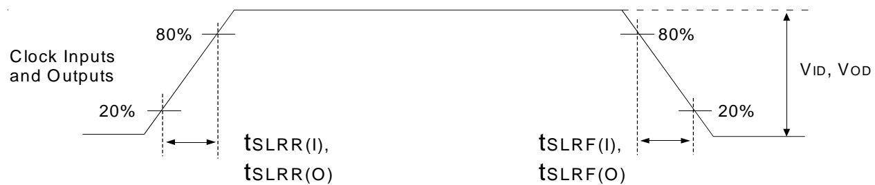
Figure 8. Input and Output Slew Rates
