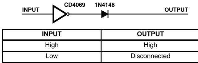
FIGURE 11A. CMOS INVERTER
