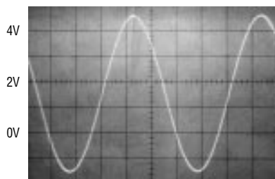
6V p-p INPUT, -1.5V TO 4.5V
