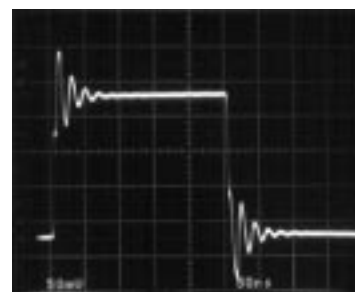
Small-Signal Transient ( A_V = 1 , C_L = 100\text{pF} )
