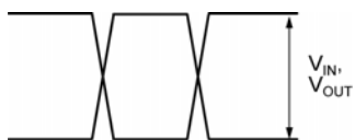
Figure 5a. Single-Ended Voltage Swing
