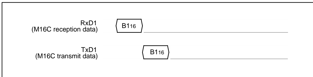
Figure 1.29.40. Timing of baud rate 19200
