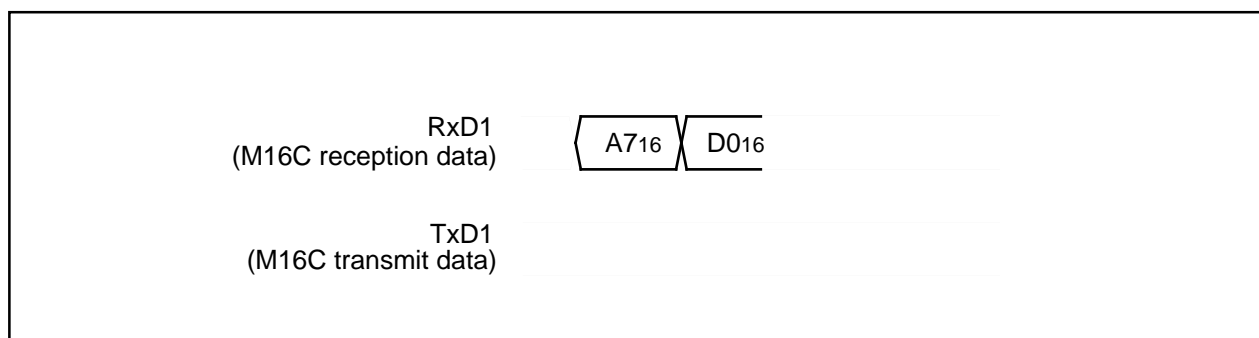
Figure 1.25.27. Timing for erasing all unlocked blocks
