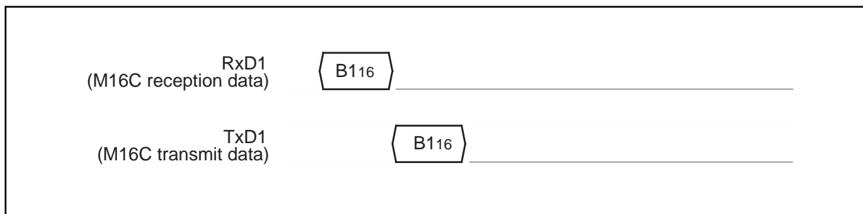
Figure 1.32.39. Timing of baud rate 19200
